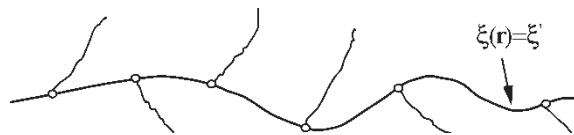
FIGURE 3 Schematic representation of Blue Moon sampling. The bold line represents the constrained ( \xi(r) = \xi' ) dynamical evolution in phase space. Open circles represent common points in configuration space which are the initial conditions of the activated trajectory sampling. Note that these points are not real crossings in phase space since the two trajectories differ in the momentum space. The dynamics represented by the light lines in the vicinity of the crossing points gives the dynamical information needed in Eq. (28).
